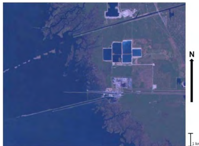
Fig. 10. Red-green-blue image of the Landsat TM data collected over the coast of Florida. This image was created with the red channel corresponding to \sqrt{(1/4)(B_3 + B_5 + B_6)} , the green channel corresponding to \sqrt{B_1} , and the blue channel corresponding to \sqrt{(3/4)B_2 + (1/4)B_4} , where B_i is the i th band of the Landsat TM image.
